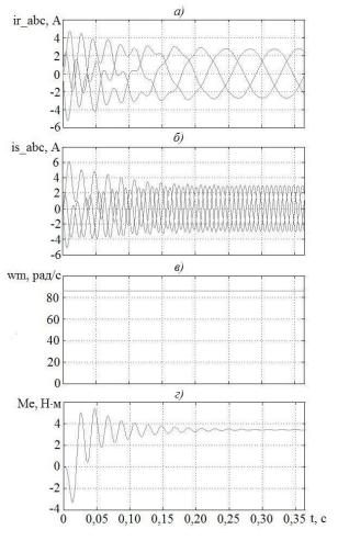
Fig. 2. Operating characteristics of the model: a) rotor winding currents; b) stator currents; c) angular frequency of the rotor rotation; d) electromagnetic torque
