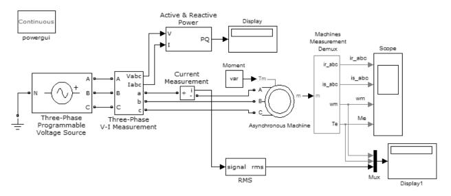
Fig. 1. Virtual model systems for research of asynchronous machine
