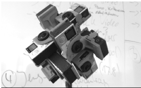
Fig. 3. Rig with mounted GoPros
