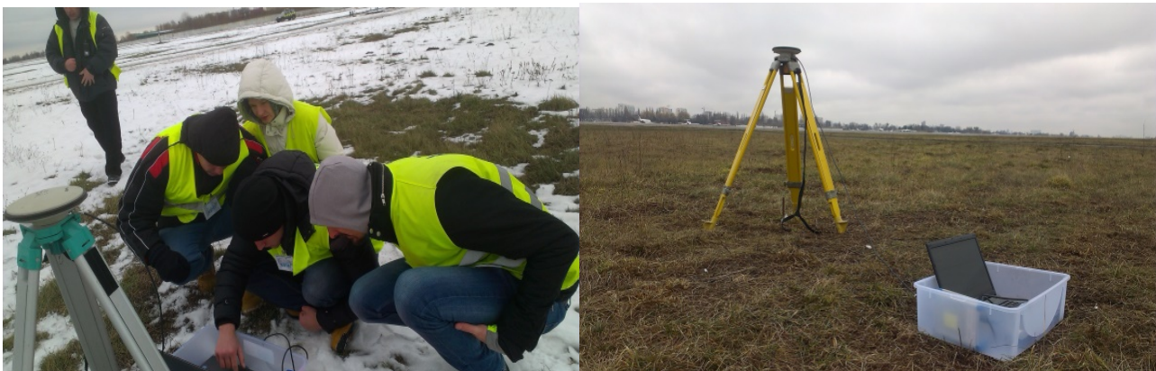
Fig. 4. Measurement equipment adjustment and GNSS data recording
