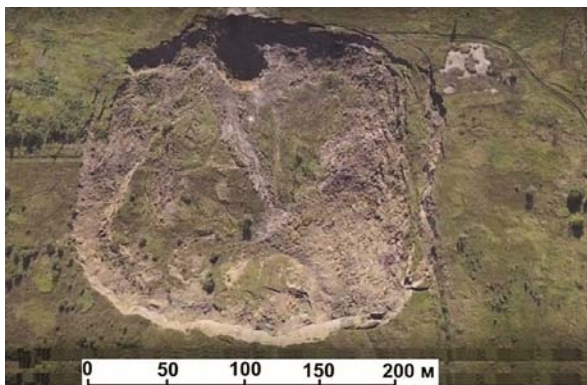
Fig. 1. Form and size of the landslide, having occurred on September 30, 2017, at the mine No. 2 [Dyakiv et al., 2019].
