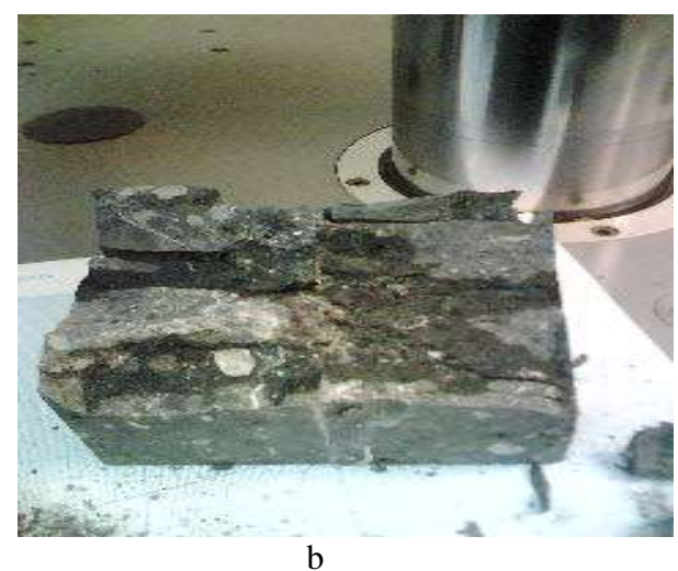
Figure 5 – Diagram of sample №5 compression (a) (Table 1) and its photo in broken condition (b)
