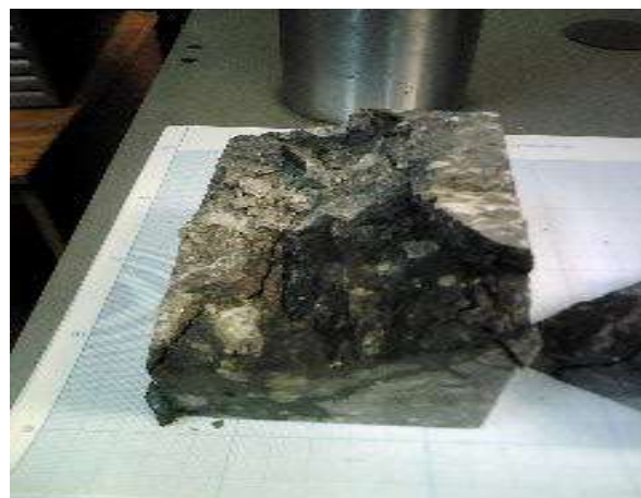
Figure 6 – Diagram of sample №6 compression (a) (Table 1) and its photo in broken condition (b)
