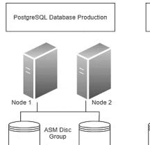
Figure 1. A schematic view of PostgreSQL databases of production and disaster were created
