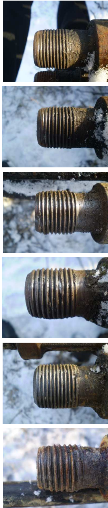
Figure 6 – Worn sucker rod thread
