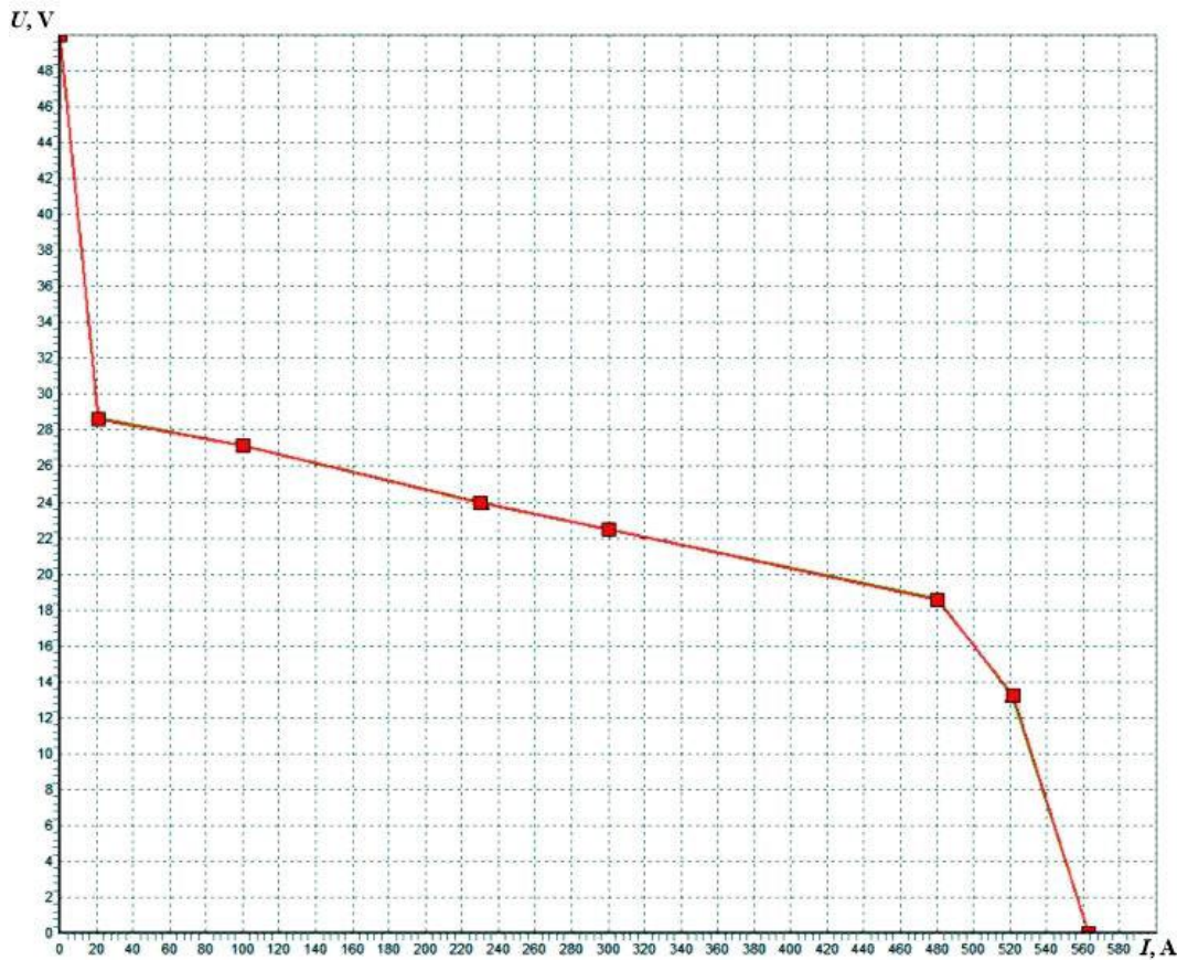
Figure 6 – Current-voltage characteristics of the power source for performing mechanized welding by a stationary process
