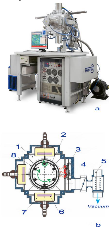
Fig. 1 – Main view (a) and schematic configuration (b) of “MVU TM-Magna 3M”. 1 – Working chamber, 2 – Planetary substrate holder, 3 – Ion-beam cleaning electrode, 4 – Throttle shutter, 5 – Valve, 6 – Target, 7 – Magnetron, 8 – Cylindrical shutter
