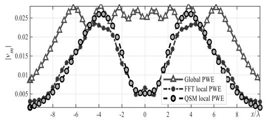
Fig. 5. Distribution of the reflected field for the transversely inhomogeneous structure.
