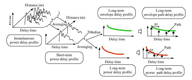
Pic 1. Features of radio waves propagation
