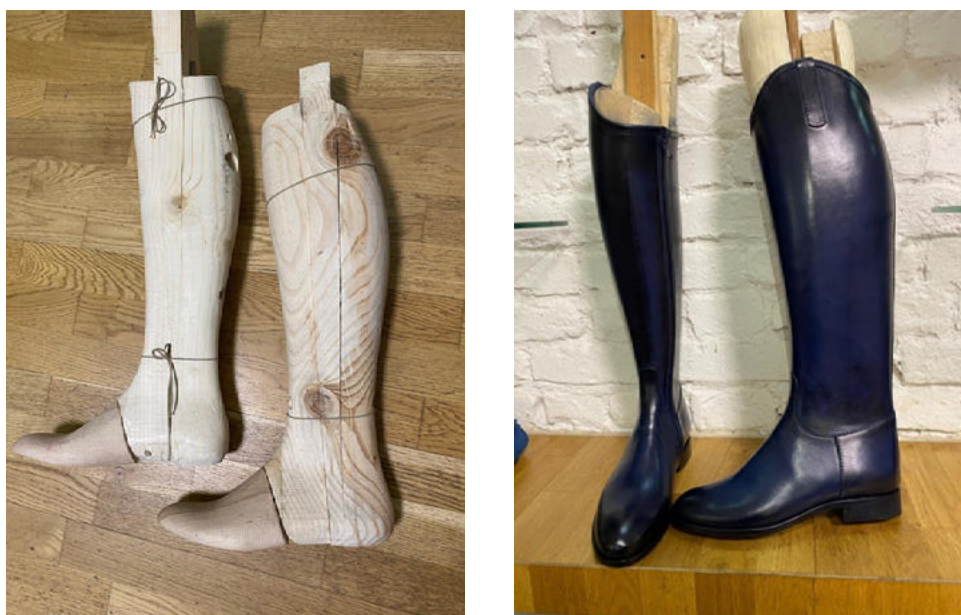
Figure 6. Assembled Mold and a Boot Made with its Help
