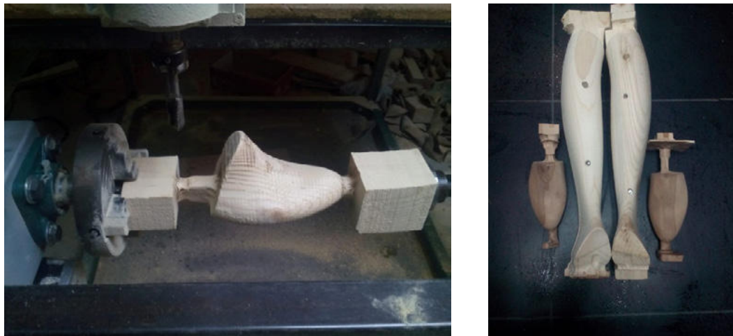
Figure 5. Production of Mold Segments on a CNC Machine
