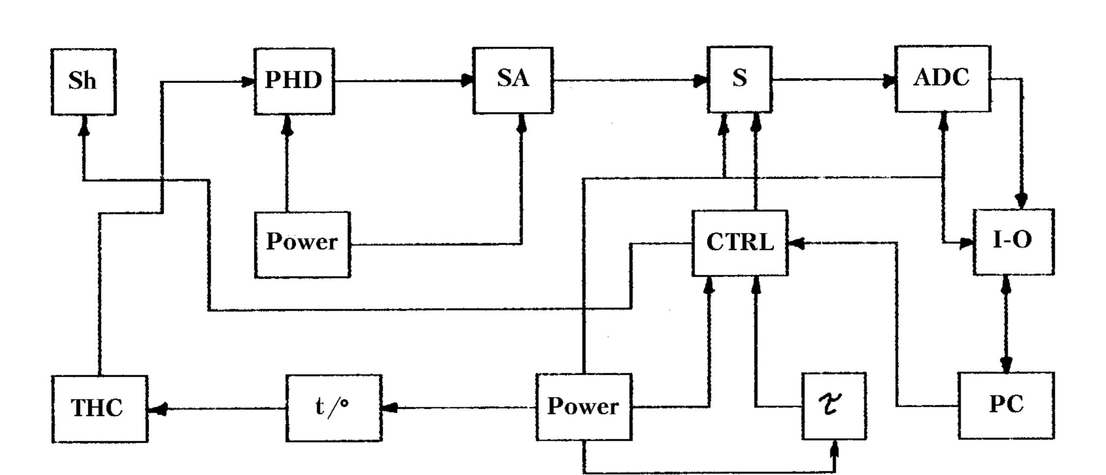
The use of the integrator (S) designed in the same series of IMS incorporating polystyrene capacitors distinguished by small current losses enables to accumulate the signal in the analog form with a sufficient precision.
