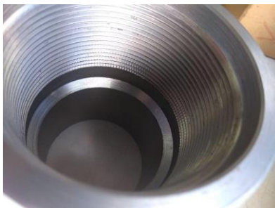
Figure 1 – Part with notches on the thread
