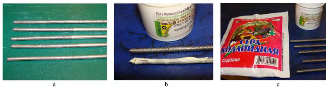
Fig. 1 – The electrodes are made of 12X18H10T (12H18N10T) stainless steel Ø 3mm intended for sulphiding the parts by EEA method
