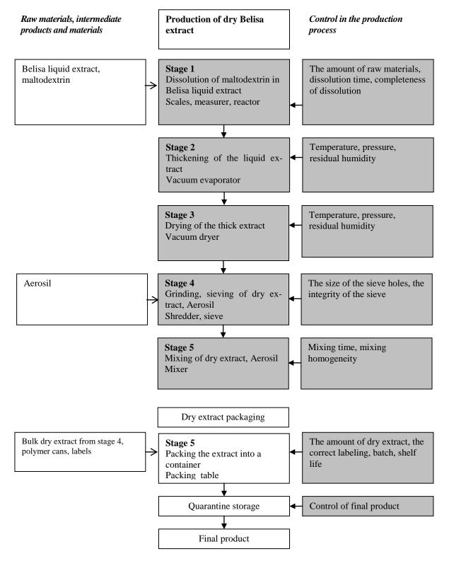
Fig. 3. Technological scheme of production of dry Belisa extract (sample No. 7)
