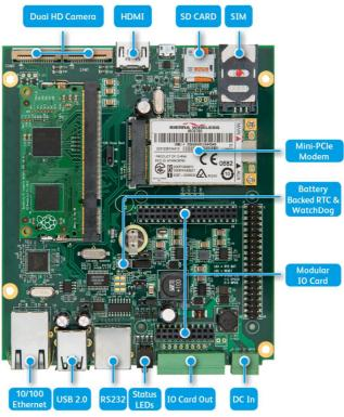
Fig. 4. Industrial IoT Integrator Board (MyPi) [6]
