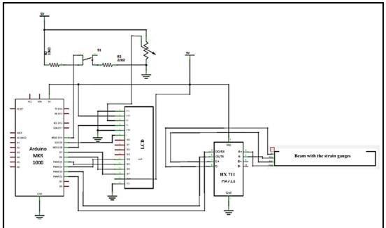
Fig. 10. Final measuring chain [16]
