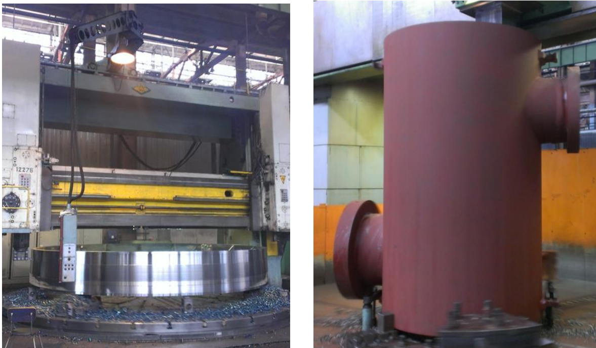
Figure 1. Heavy duty housing workpieces processed by heavy duty vertical turning and boring mills on the sites of the „EMSS“ and the „NKMZ“ Public Companies
