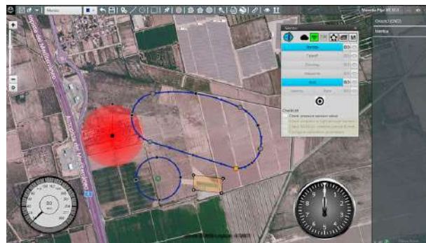
Figure 9. Tools for creating a flight plan in the onboard FC «Veronte Air»
