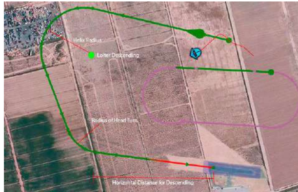
Figure 16. Tools for additional maneuvering of the UAV before its arrival on the runway
