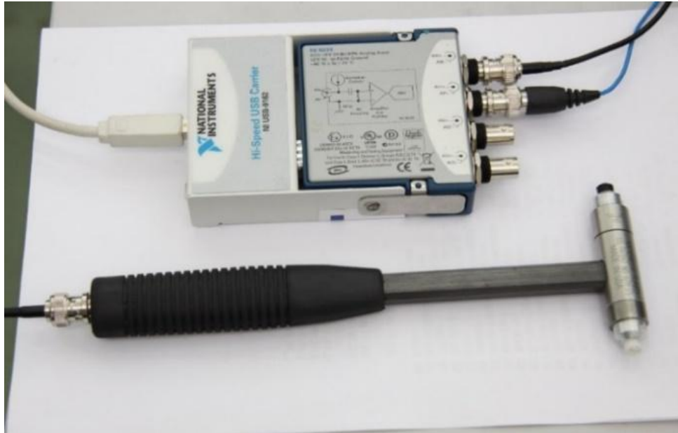
Fig. 1. Strike hammer of M355B15 model made by PCB firm
