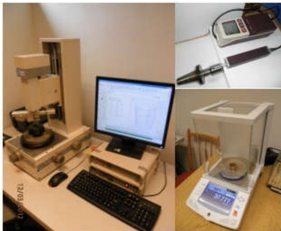
Fig. 3 – Devices used: MUK – F 300 PC, Mitutoyo SJ-201 and Voyager Pro VP 613 CN
