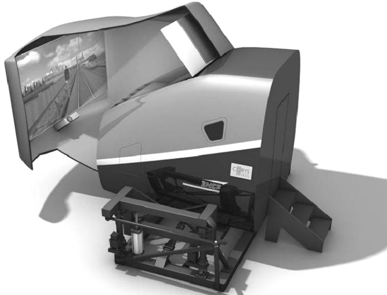
Fig. 1. General view of a full scope cab replica simulator on a motion base
