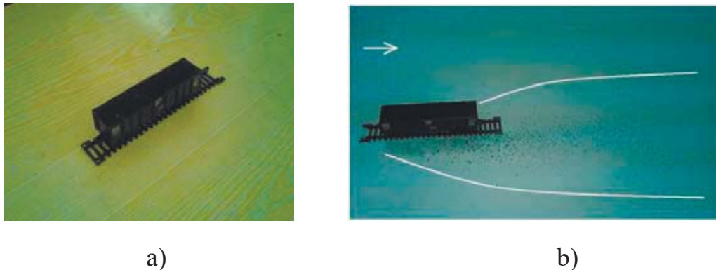
a) Model of poorly loaded wagon; b) Contaminated zone (abrupted) near poorly loaded wagon.
